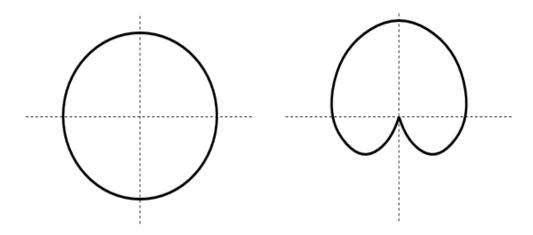
Figure 20. Omnidirectional (left) and cardioid (right) microphone polar patterns.
