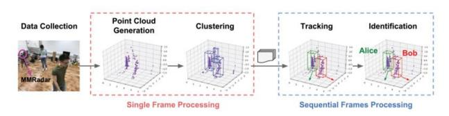
Figure 24. Point Cloud Example of two persons detected by an mmWave radar (image from [III.76])
