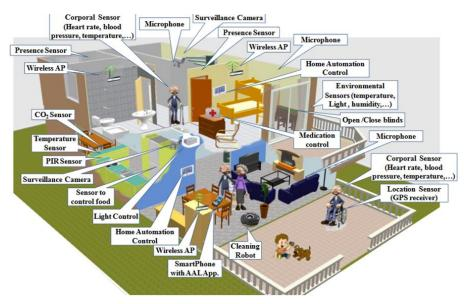
Figure 7. An example of the various types of sensors that could be deployed in a house or assisted-living environment (reprinted from [II.23])
