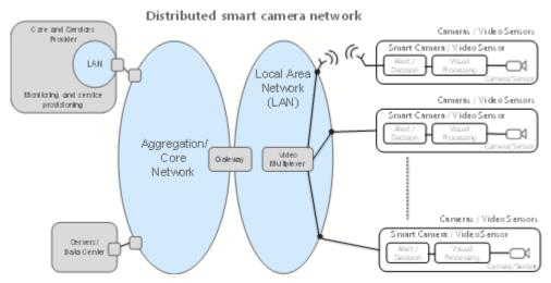
Figure 37. Distributed smart camera network
