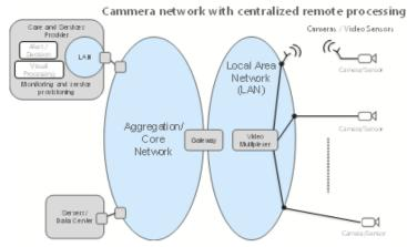
Figure 35. Camera network with centralized remote processing
